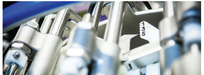
BAADER evisceration machines can easily be adjusted to fit the flock size Picture Courtesy: BAADER
