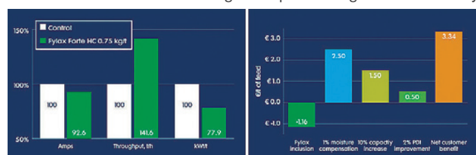
Fig. 1: Relative effect of Fylax Forte HC in a 10% hydrating solution on pelletiser specs (based on 8 commercial trials)
