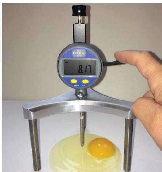
Fig. 4: The Haugh unit (pronounced: “how”) is a widely recognised measure of an egg’s internal quality and freshness
