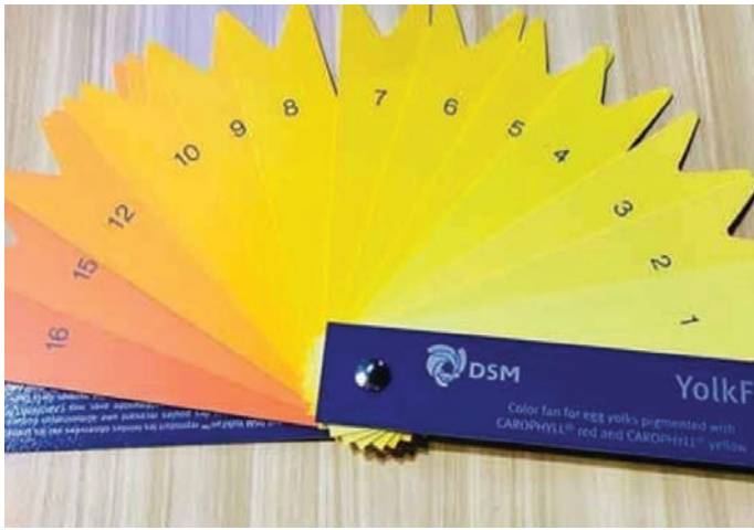
Fig. 5: The Yolck Fan, made for assessing egg yolk colour to monitor chicken nutrition
