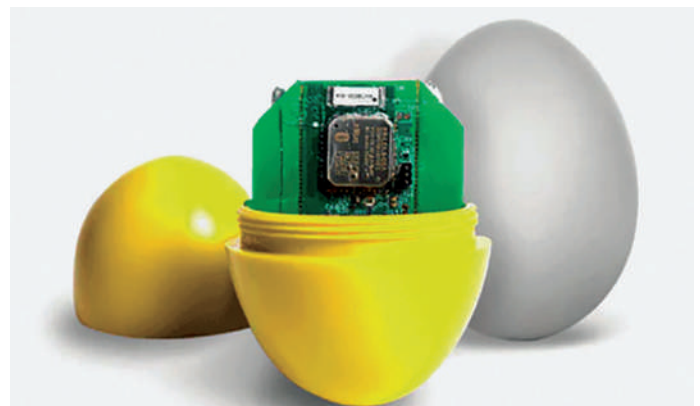
Figure 2: An artificial egg with a G-force sensor inside
