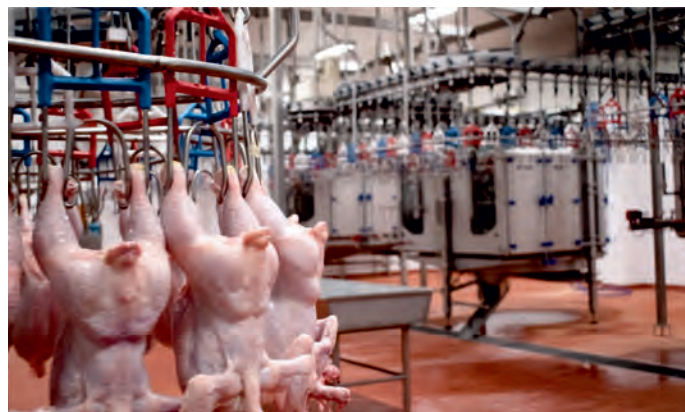
Evisceration equipment should be adjustable to fit the flock size being processed to protect the product quality and minimise contamination.
